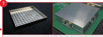
You now have a finished can! Use the can with S1711-46R RFI Shield Clips provided.
