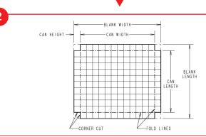
Use this diagram as a guide when cutting your etched Shield Can Sheets.
