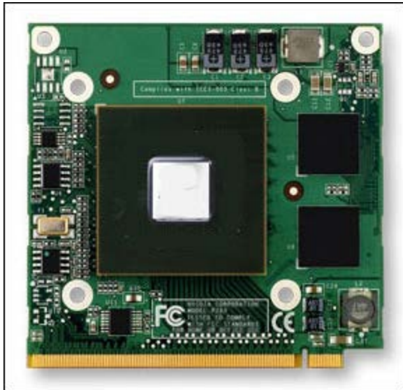
Figure 1. An MXM GPU, showing the standard MXM connector pins at the bottom edge.
