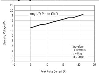
Clamping Voltage vs Peak Pulse Current
