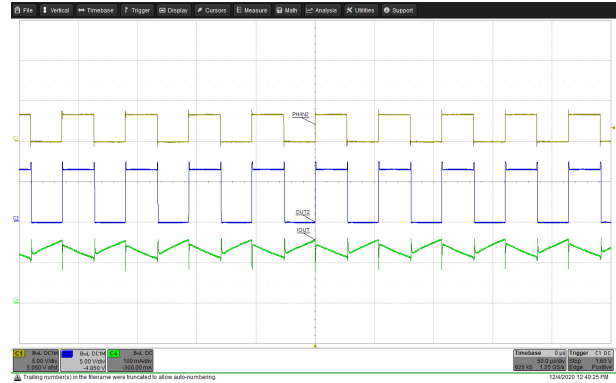
A. Channel 1 = IN2 Channel 2 = V_{OUT2} Channel 4 = Motor Current
