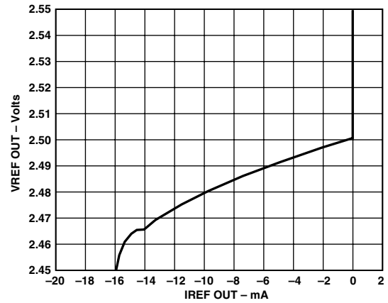
TPC 23. Reference Voltage vs. Reference Load
