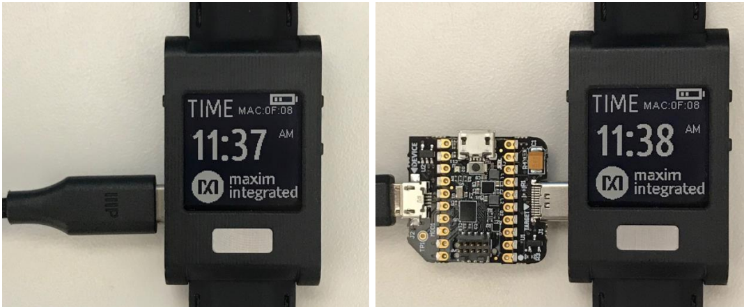
Figure 14. USB connection to PC using a USB Type-C cable (left) and Pico adapter board (right).
