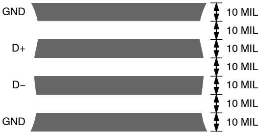
Figure 22. Arrangement of Signal Tracks
