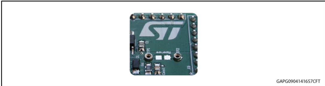
Figure 4: Mounting through-hole sense resistor
