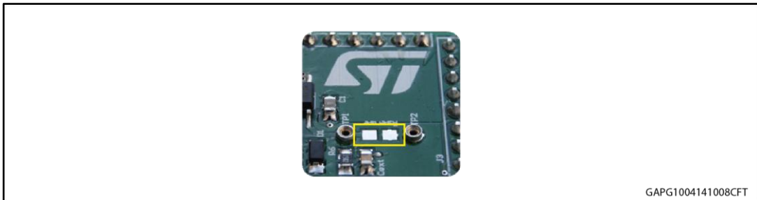
Figure 5: Pads for soldering SMD resistor
